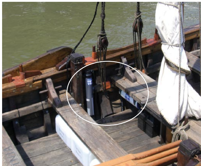
Top: The replica of John Smith's shallop at dock. Above: The underway monitoring system, including a YSI water quality sonde, discreetly mounted aboard the shallop.
